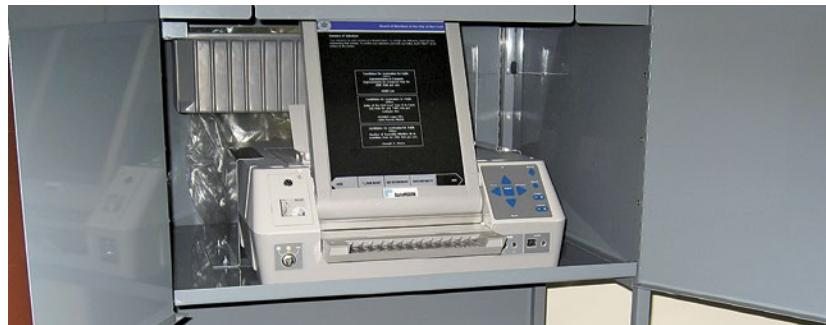
16. Open the ballot feed tray that is in the front of the BMD, by pulling up on the top and then outward away from the BMD.
