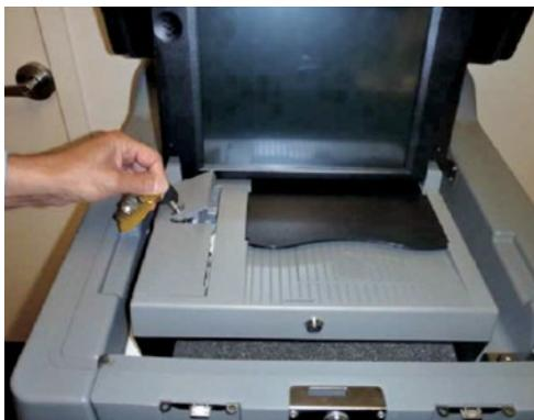
**1.** Break the yellow seal and open PMD Compartment Door (Location #1) with barrel key from Scanner Police Envelope.
