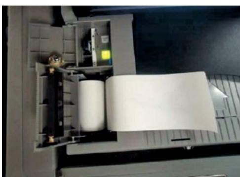
**5.** Put the new paper roll (side with scratch mark) down.
