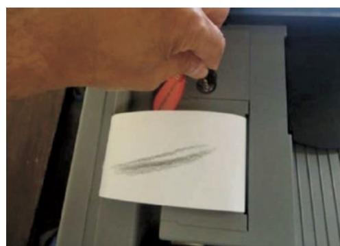
**6.** Close the paper compartment door and turn the key to lock. Do not place a new seal on door.
